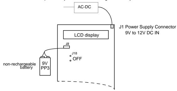
Figure 2-3. C51/C251 Demo Board powered by J1 with a rechargeable battery on J2
